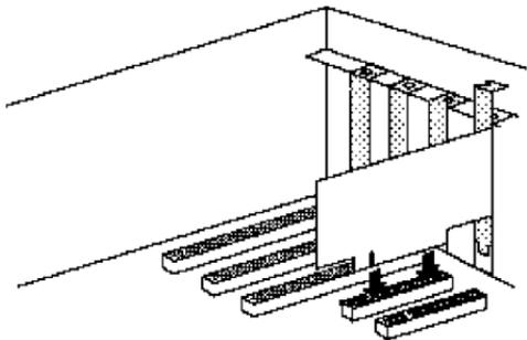
6. Secure the card using the screw that you removed previously.
